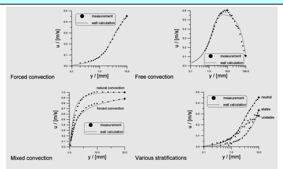
Velocity distribution results of the wall calculation in comparison with experimental data
