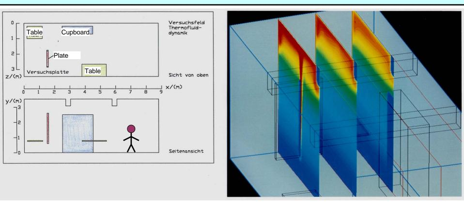
Comparison of the heating power of the vertical plate in the lab.
